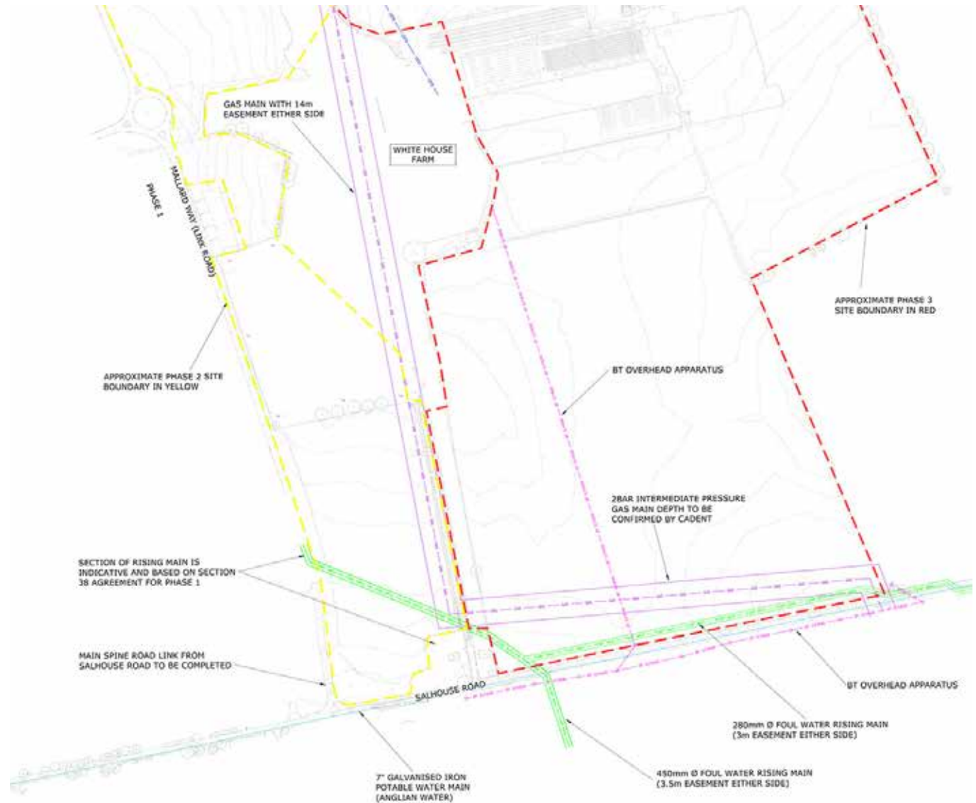
Figure 21: Extract from Richard Jackson report: Existing utilities - southern section of the site
