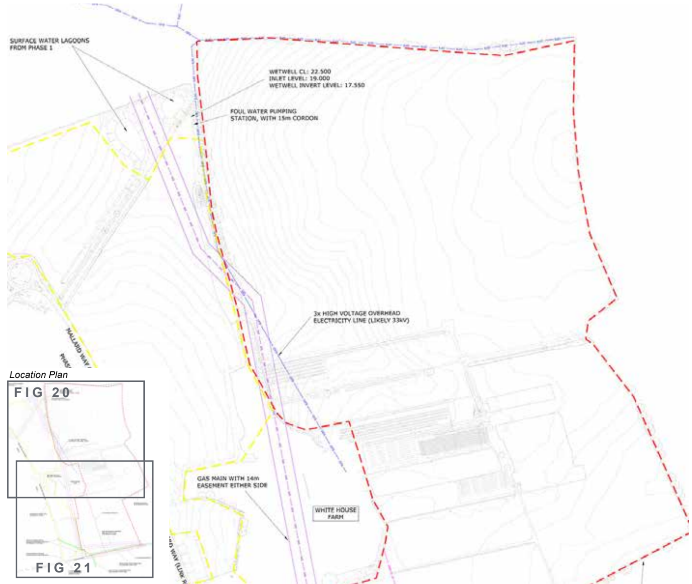
Figure 20: Extract from Richard Jackson report: Existing utilities - northern section of the site
