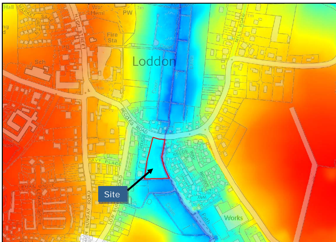
Figure 3: Filtered LIDAR survey of the site and surrounding area combined with OS (where low ground is denoted by blue colours and higher ground is denoted by green and yellow colours)
