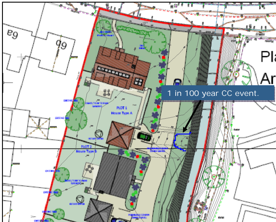
Figure 9: Extent of Upper End climate change 1 in 100 year event in relation to proposed layout
