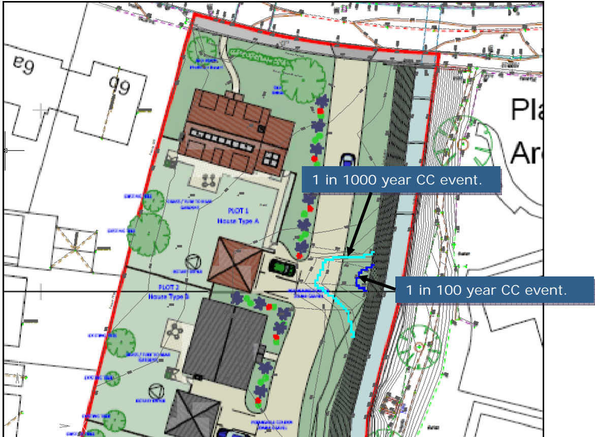
Figure 8: Climate change 1 in 1000 year extent and climate change 1 in 100 year (Higher Central) 1 in 100 year extent in relation to proposed layout
