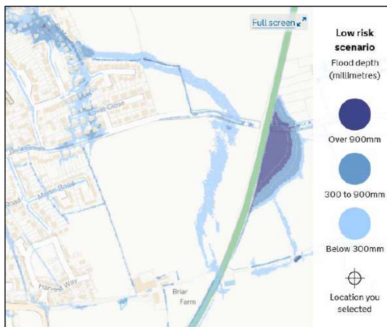
Surface water flood map extract (02/11/2018)© Crown copyright and database rights 2018 Ordnance Survey 100047325
