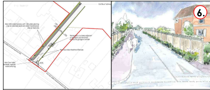
SECONDARY ACCESS: SECONDARY ACCESS POINT ALLOWING FOR EMERGENCY VEHICLE ACCESS AND A FOOTPATH LINK TO THE NEW SCHOOL ENTRANCE AND RESIDENTIAL DEVELOPMENT
