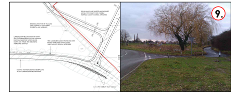
PRIMARY ACCESS: MODIFIED JUNCTION ARRANGEMENT ONTO BURGH ROAD, DIRECTING TRAFFIC AWAY FROM SIR WILLIAM'S LANE INTO THE DEVELOPMENT SITE
