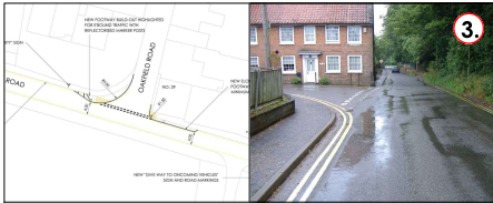
BURGH ROAD SHUTTLE WORKING: LOCALISED TRAFFIC CALMING SCHEME ALSO ALLOWING WIDENING OF EXISTING NARROW SECTION OF FOOTWAY ON EAST SIDE OF JUNCTION
