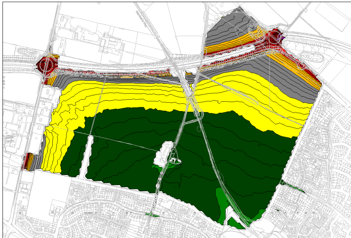
Figure 2: Night-time Noise Levels With Proposed Noise Bund
