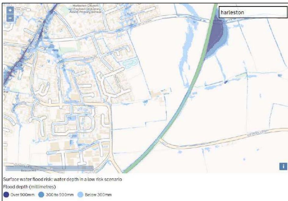
Surface water flood map extract low risk flood depths (13/03/2020)© Crown copyright and database rights 2020 Ordnance Survey 100047325
